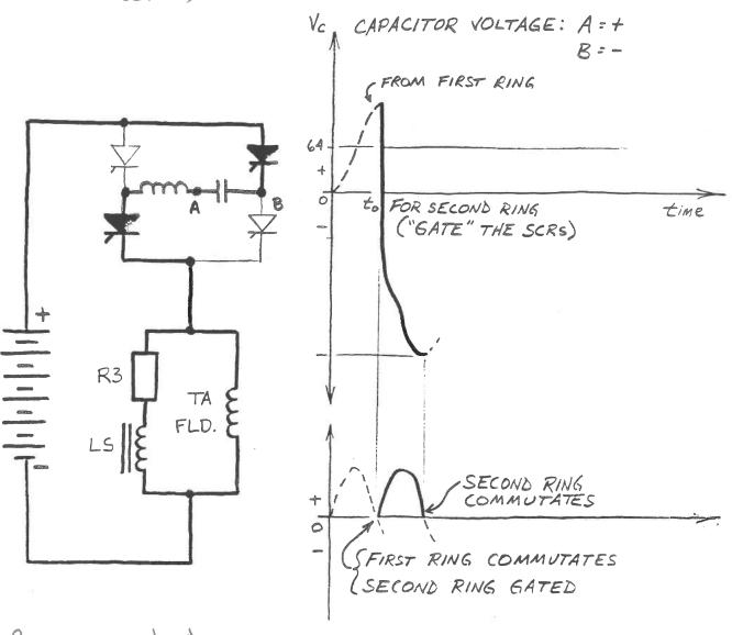
Reverse polarity in capacitor and double its voltage to 2000
