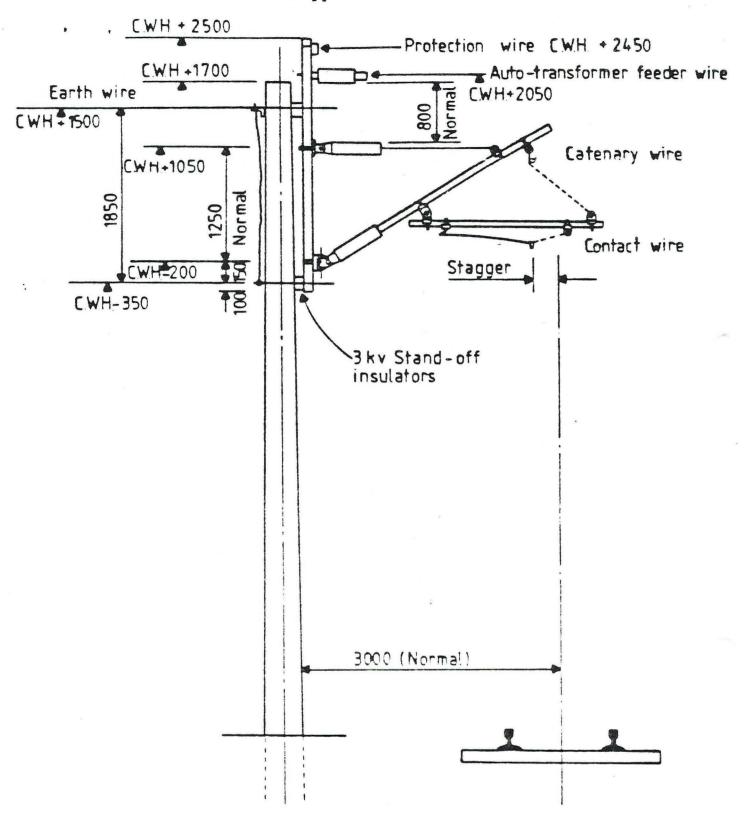
Maximum stagger - Tangent track - 200 mm Maximum stagger - Curved track - 250 mm, All staggers to be set to minimise mid-span offset
