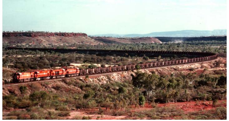
A loaded (240-car) iron ore train climbs the 1 in 50 grade through the Chichester Range in the pre-GE days. Of interest is the fact that the lead unit of this lengthy train is 14 metres higher than the last car of the consist 2.6km back down the grade. Bob Hepburn
